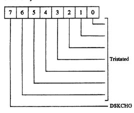
When the Digital Input Register (DIR) is in PC/AT mode, only bit 7 (DSKCHG) is driven. Bits 6:0 are tristated to avoid conflict with the fixed disk status register at the same address. The DSKCHG bit monitors the pin of the same name and reflects the opposite value seen on the disk cable. Bit 7 is forced inactive along with the inputs from the floppy drive, while the other bits remain tristated. The Digital Input Register is unaffected by a software reset.
