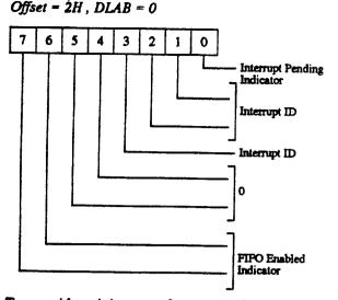
To provide minimum software overhead during data character transfers, the UART prioritizes interrupts into four levels and records these in the Interrupt Identification Register (IIR). The four levels of interrupt conditions in order of priority are
