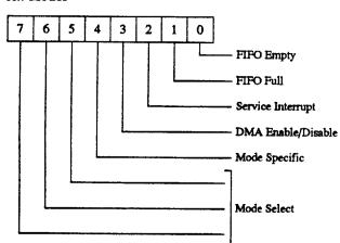
The read/write Extended Control Register (ECR) controls the extended parallel port functions and is always accessible.
