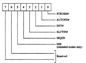
The read/write Control Register (DCR) provides all output control signals to the printer.
