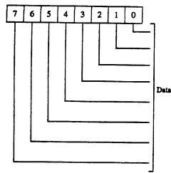
The eight-bit read/write Mouse Port Data Register transfers data between the host and the mouse. The host sends command and data bytes to the data register on the MDATA line, using the MCLK as the synchronizing signal. The register converts status and other data from the mouse into 8-bit bytes and transfers the data to the host via the seried MDATA line.
