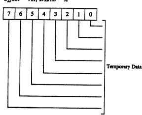
This eight-bit register does not control the UART in any way. Its purpose is to hold data temporarily.
