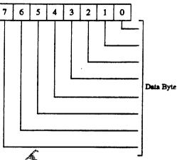
This register holds the data byte to be sent to the host. Bit 0, the Least Significant Bit (LSB), is transmitted first. The data is loaded into the Transmit Shift Register (not user "accessible) from the Transmit Register or Transmitter FIFO. This byte is then transmitted to the TXD pin.
