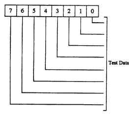
TheTest FIFO (tFifo) transfers 8-bit programmed I/O or DMA test data to and from the system. FIFO data is not relayed to the parallel port lines with a hardware protocol handshake.
