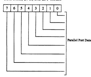
The parallel port Data Register (DATA) is a bidirectional, 8-bit data port. Data written to this register is transmitted to the printer; data read to it is the data on the connector. This port is 100-percent compatible with the IBM PC/AT parallel port. STATUS REGISTER Read Only Byte at LPT +1H in All Modes
