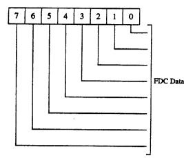
All command/status parameter information and disk data transfers go through the Data Register or FIFO. The data transfers are controlled by bits D7 (RQM) and D6 (DIO) in the Main Status Register. The FIFO is 16 bytes and basprogrammable threshold values.
