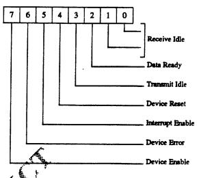
Device Enable. The host sets this bit to 1 to enable clocking to the pointing device. A 0 disables clocking to the pointing device. This bit must always be enabled when the mouse is in use.
