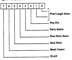
The Line Control Register (LCR) is used to specify the format of the asynchronous data communications exchange and to set the divisor latch access bit.
