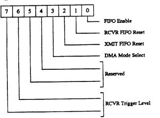
This write-only register is at the same location as the Interrupt Identification Register, a read-only register. The FIFO Control Register is used to enable the FIFOs, clear the FIFOs, set the RCVR FIFO trigger level, and select the type of DMA signaling
