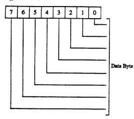
Add the isolation of th This register holds the incoming data byte. Bit 0, the Least Significant Bit (LSB), is received first. The data is initially assembled in the Receiver Shift Register (not user accessible) before it is loaded into the Receive Buffer or Receiver FIFO.
