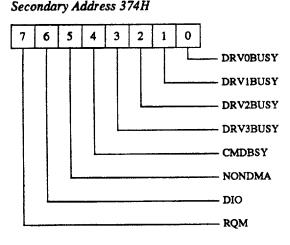
The Main Status Register (MSR) is always available to be read. The MSR is used for controlling command input and result output for all commands. It gives the current status of the FDC, and indicates when the disk controller is ready to send or receive data through the data register (FIFQ)
