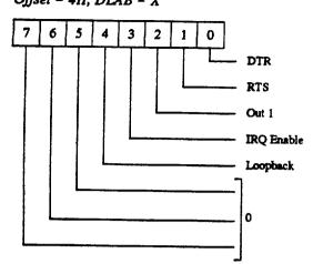
This register controls the interface with the modern, data set, or peripheral device emulating a modem.
