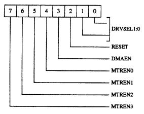
The Digital Output Register (DOR) controls the drive select and motor enable disk interface outputs, enables the DMA logic, and contains a software reset bit. The content of the DOR is set to 00H after a hardware reset and is unaffected by a software reset. The DOR can be written to at any time.
