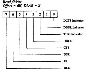
The Modem Status Register (MSR) provides the current state of the control lines from the modem or peripheral device to the CPU. In addition to this current information, four MSR bits provide change information. These bits are set to logic 1 whenever a control input from the modem changes state. They are reset to logic 0 whenever the CPU reads the MSR.
