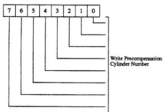
This register is written to by the host. It usually contains the number of the cylinder where the write precompensation is to be used.
